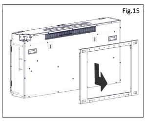
15. The Fire (G) is also supplied from the factory with 4x or 6x finger bend fixing brackets. Lay the Fire (G) on its back again. Each bracket is held in place with 2x screws. Remove all brackets. They are not required for this installation. **Fig. 13-16**.
