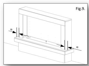
9. Mark a line under both pre-installed L-brackets 10mm in from the MDF side blocks. **See Fig.10.**
