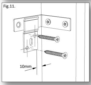
11. Securly fix the Wall Brackets (C) In place, on each side of the Mount Board (H). **See Fig.12**.
