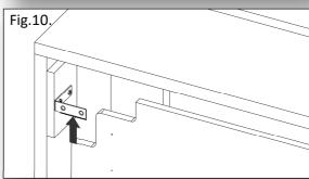
10. Position the 2x Wall Brackets (C) on the wall markings as detailed. **See Fig.10,11**.
