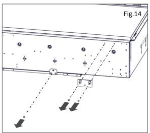
14. Position the Fire (G) back on to its base and angle the wall mount bracket away from the Fire (G) at the base, then move the bracket down off the hook points. **Fig.15.**
