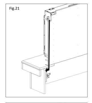
21. Peel the film off the adhesive tape on the rear of the mood lighting and adhere to the **polished** face of the plinth under the Hearth top.
